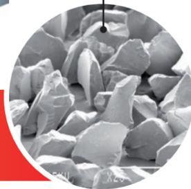
Conventional ceramic abrasive grain is irregular in shape. Instead of a clean, machining action, the grain “plows” through the metal, causing heat build up, slower cutting and shorter life.
