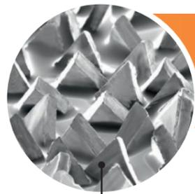
The triangular ceramic abrasive grains are easily detectable under a microscope. 3M capitalize Precision-Shaped Grain in Cubitron II vitrified wheels continuously fracture to form sharp points and edges-slicing cleaner and faster, staying cooler and lasting many times longer.
