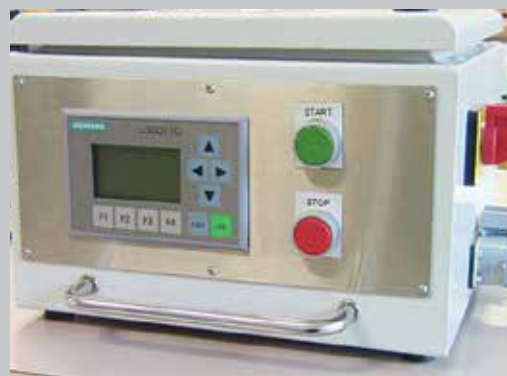
SBA control box automatic for time-regulated cut-in-finishing of individual parts and small series
