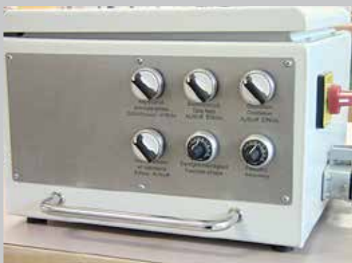
SBM control box manual for manual finishing of individual parts and small series
